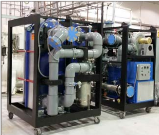
Heat Exchanger, Condenser, CO 2 Addition, Heater, Blower,
